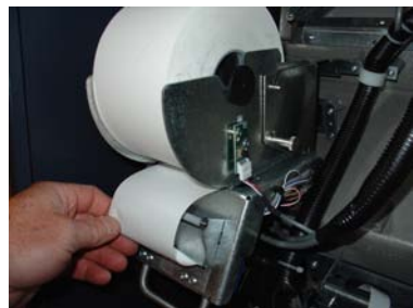
Figure 6-6. Feed paper into slot.
