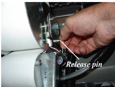
Figure 6-8. Release pin location.
