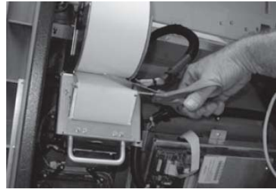
Figure 6-1. Cut paper between the roll and input to the printer.
