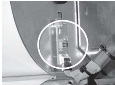
Figure 6-2. Paper feed button is located on the paper bracket.
