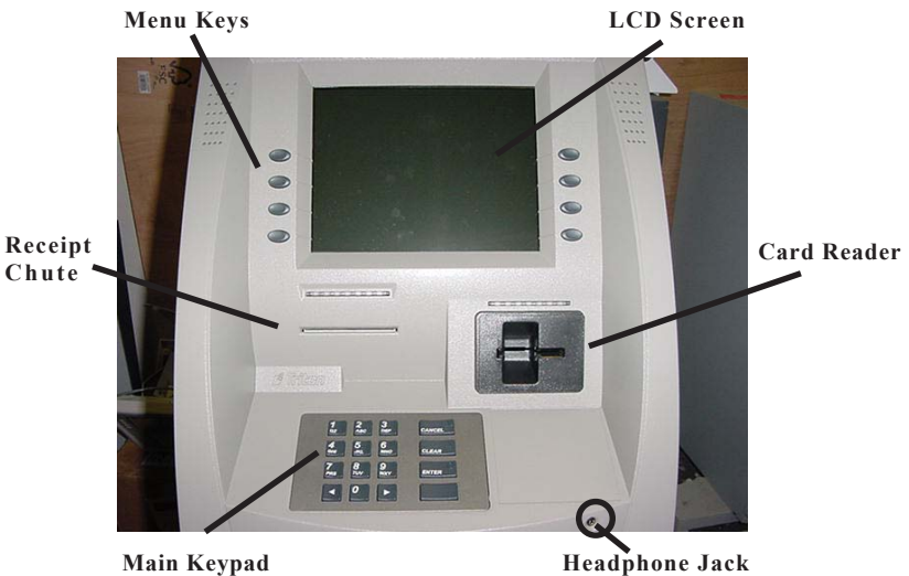
Fig. 2-1. Control panel layout
