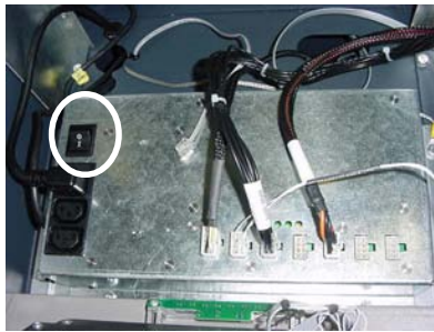
Fig. 7-9. Power supply ON/OFF switch location.
