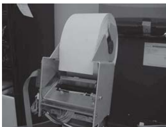
Figure 6-6. Paper feeds from top of roll.
