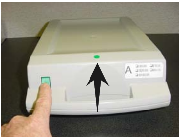
Press release button and lift top.
