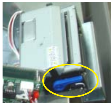
Blue tension lever (correct position).
