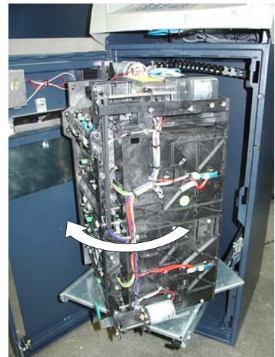
Rotate turntable “clockwise”.
