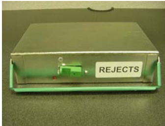
Lockable reject vault.
