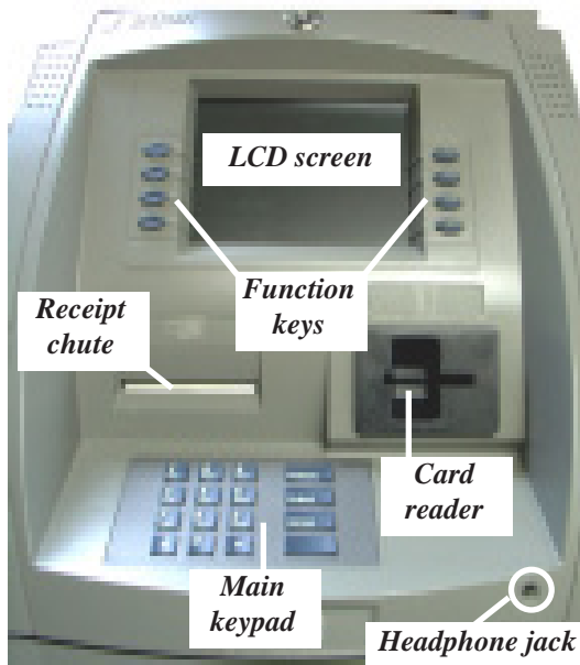
Figure 2-1. Control panel layout.
