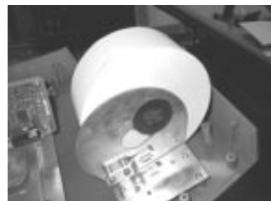
Figure 6-5A. Placing the paper roll and spool on the paper bracket.
