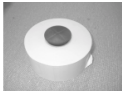
Figure 6-4B. Spool inserted into the roll of paper.
