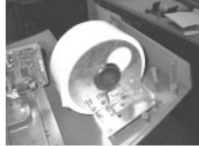
Figure 6-5B. Paper roll and spool in place for operation.
