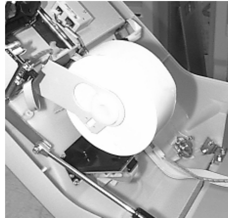
Figure 6-6B. Paper roll and spool in place for operation.
