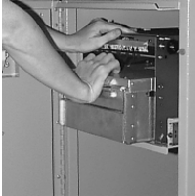
Figure 4-8. Installing the cassette into the dispensing mechanism.
