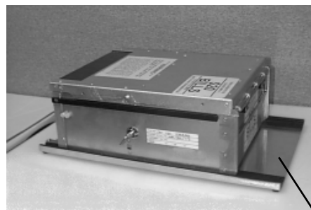
Figure 4-4. Currency cassette on a loading tray. LOADING TRAY
