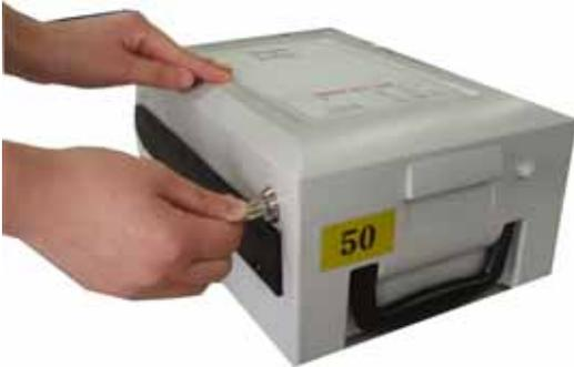
6) Close the cassette cover and turn the cassette key counter clock-wise until it is locked. Remove the key when it is locked.
