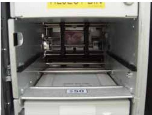
6) Remove the jammed note inside CDU body carefully .
