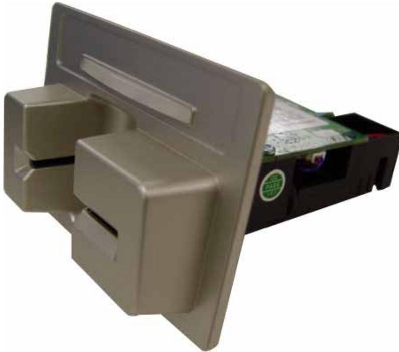
Fig. 3.7 MCU (Magnetic Card Unit)
