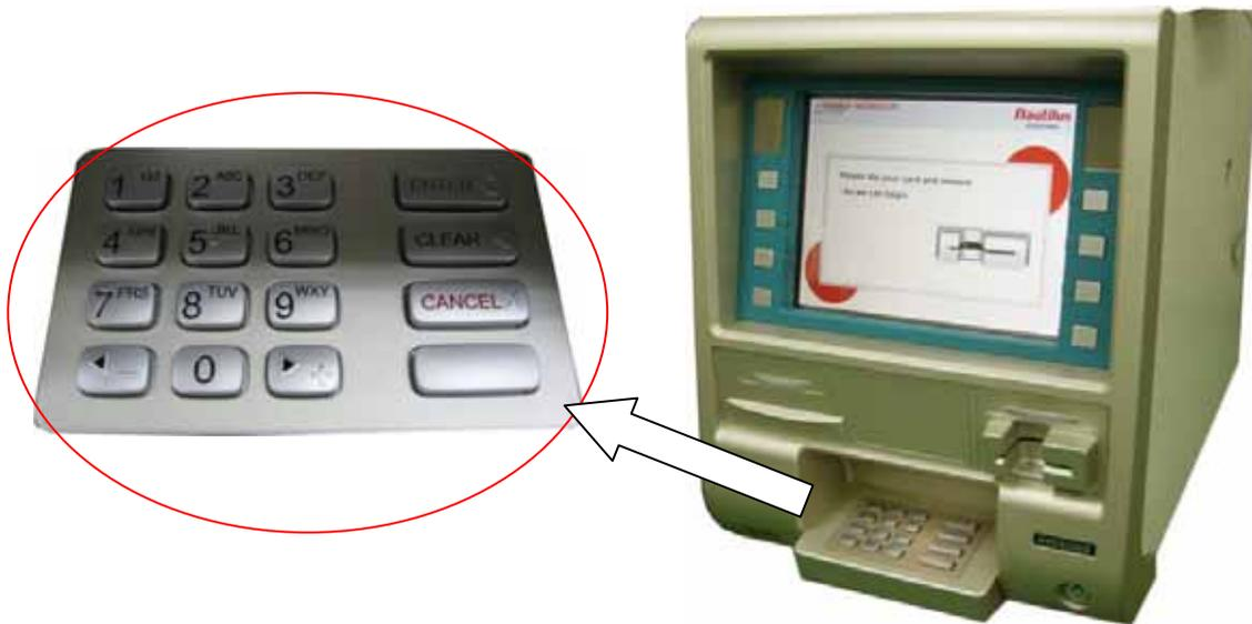
Fig. 3.3 Display for customer and keypad
