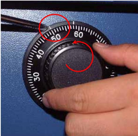
**Note:** The left scale mark is used to change the combination.
