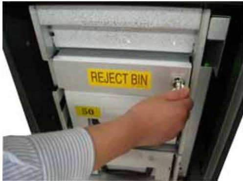
1) Insert the reject box key, turn it clockwise
