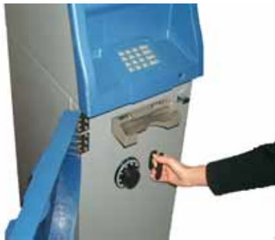
Fig. 5.3a Replenishing the Cash Cassette
