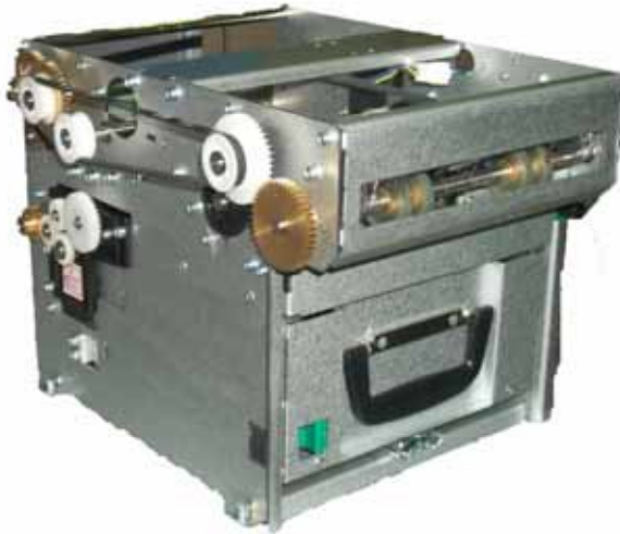
Fig. 3-4 Cash Dispenser Unit
