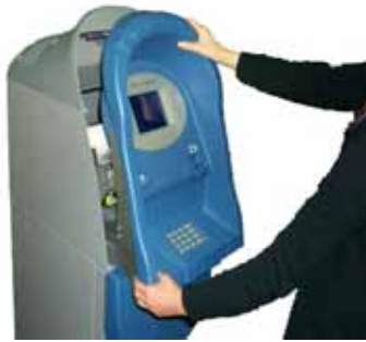
Fig. 5.2a Opening the Front Panel
