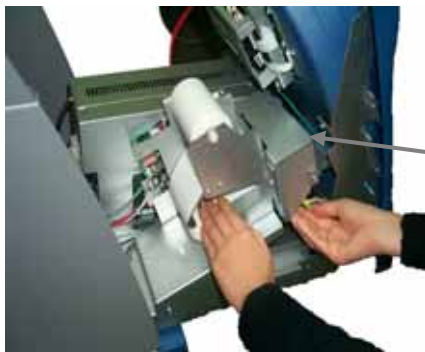
Fig. 5.5a Loading the Receipt Paper
