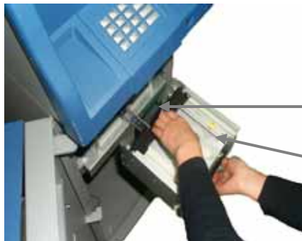
Fig. 5.3a Replenishing the Cash Cassette
