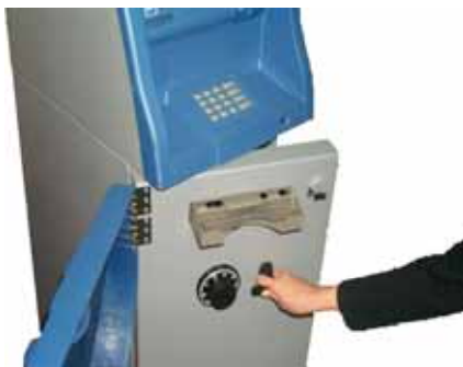
Fig.A-1 Opening the Security Door
